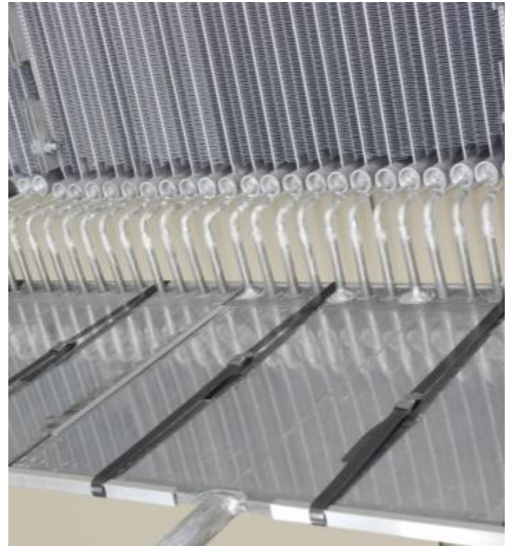
Connection between Bionic Distributor and MPE-tubes.
